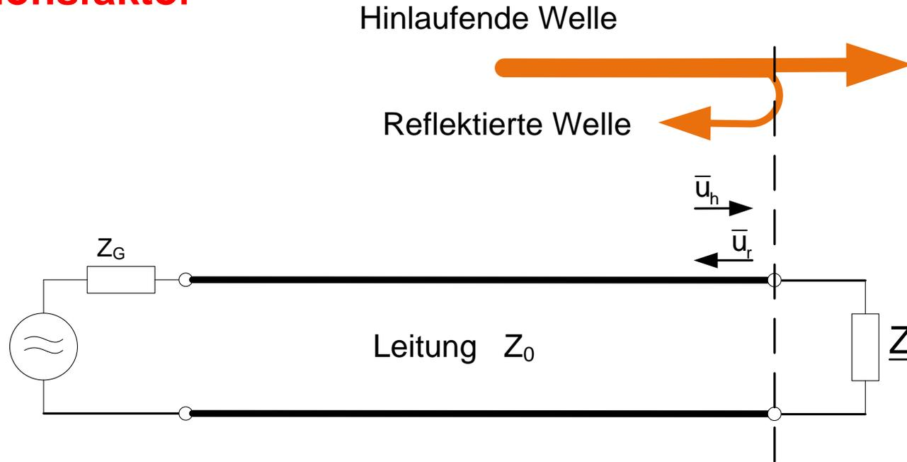
$\underline{\Gamma}$  : Komplexer Reflexionsfaktor =  $|\Gamma| \angle \theta$        $\underline{\Gamma} = \frac{|u_r|}{|u_h|}$
