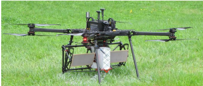
Gamma S-Band SAR (GSSAR) on Harris HX8 UAV Gamma L-Band SAR (GLSAR) on Harris HX8 UAV
